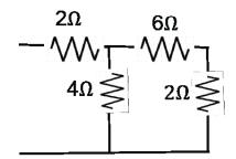
Step 3: combine  $2\Omega$  and  $6\Omega$  resistors [series]:  $2\Omega = 6\Omega = 8\Omega$
